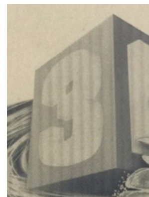
CONVENTIONAL: Flute marks highly visible
