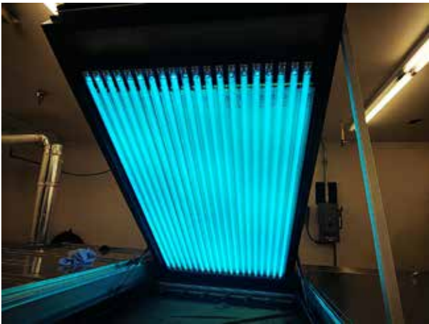
Inline-UV post-exposure ensures high plate uniformity
