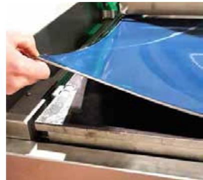
Magnetic sticky table is easy to replace
