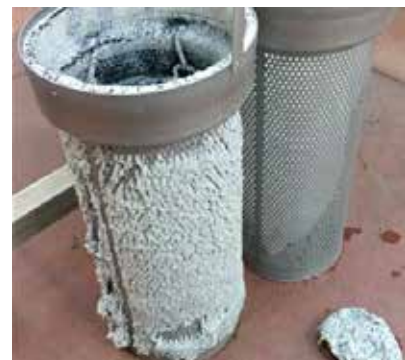
Filter cartridges for easy to replace polymer filter waste
